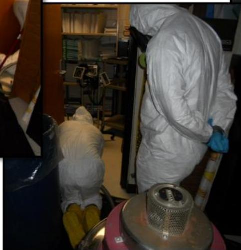
Mercury Recovery Vacuum in use.
