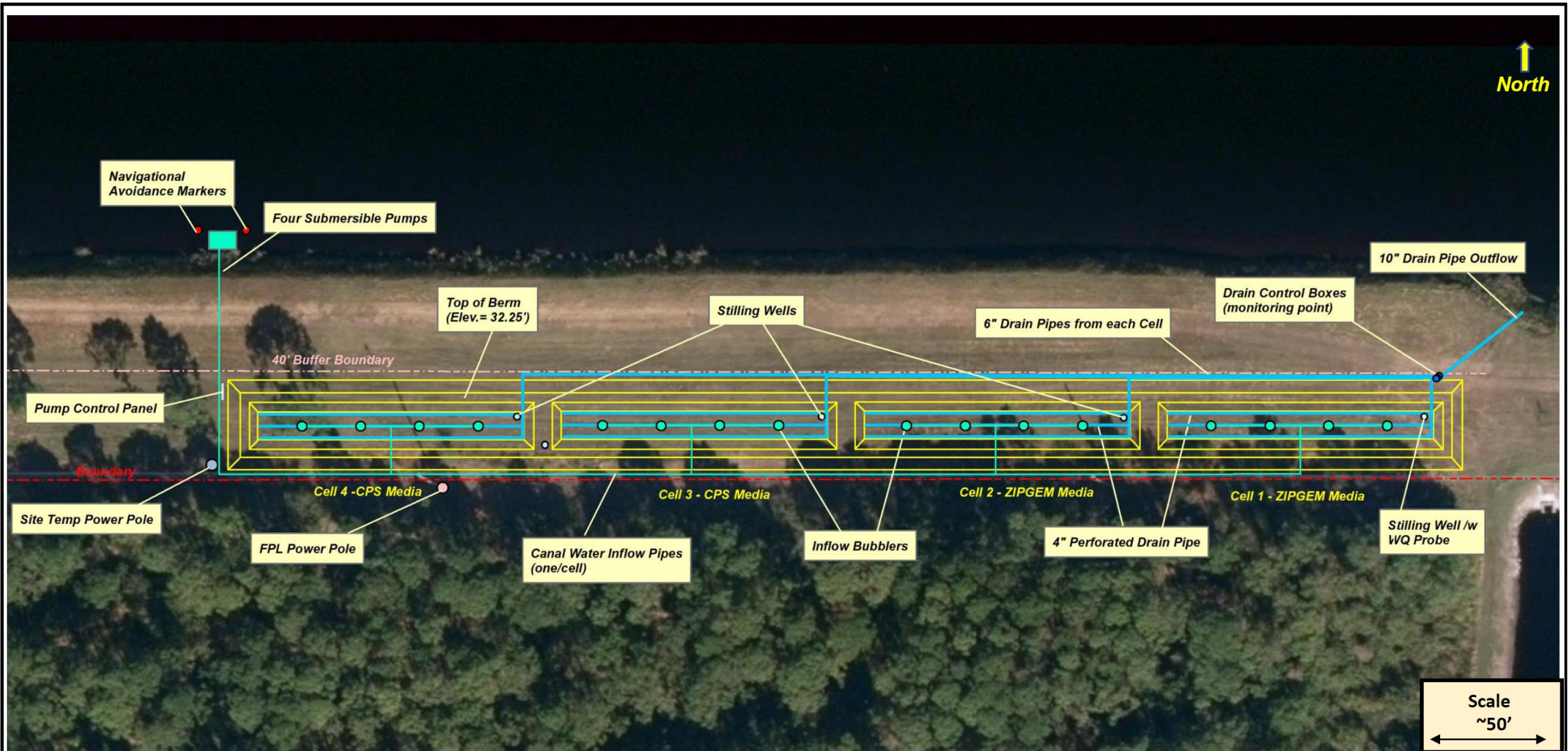
Sheet 2. Site Layout with Drain Control Boxes Together at Outlet
