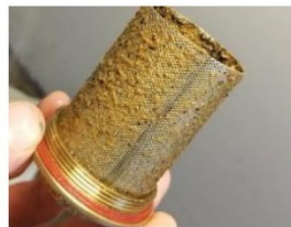
Reduced Flow and Blockages
