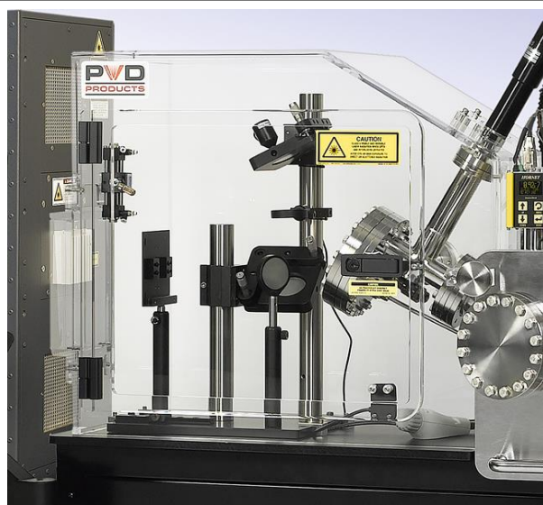
PVD Products enclosed optical train with shutter, XY aperture, focus lens and mirrors. Also seen is the raster actuator and Intelligent Window described below
